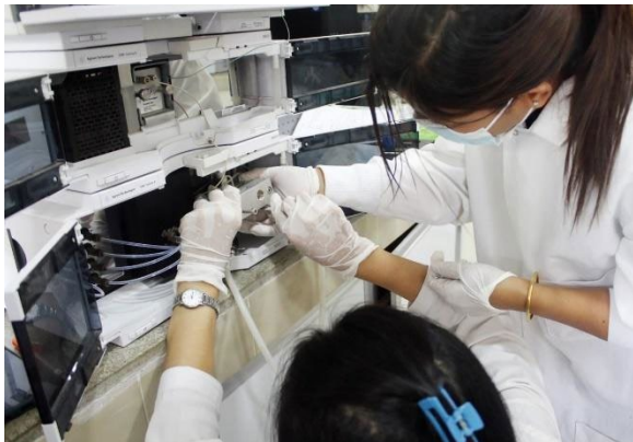
Left: Analysts at DFDA Nay Pyi Taw Pharmaceutical Chemistry Laboratory perform preventive maintenance of an HPLC system during metrology training. Right: A subject matter expert from PQM+ remotely delivered the measurement uncertainty training through Microsoft Teams while an in-country consultant facilitated the learning activities and hands-on sessions in the laboratory.
